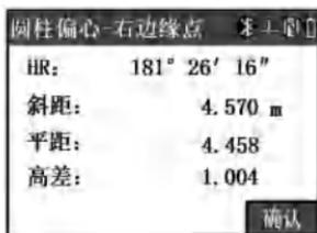
瞄准左边缘后按[确认]键，进入“圆柱偏心-右边缘”窗口，瞄准右
